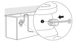
2 Remove the knockout plug **1** from the disposal.
