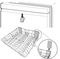
• Press the tab to remove the cable tie by hand. Cutting the tie with a knife or scissors may damage the rack or the silverware basket.
