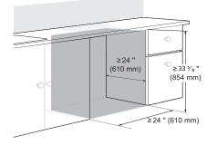
2 To allow for proper clearance of plumbing and electrical, use the template included with the literature to determine the clearance on the side of the cabinet where the cabinet meets the back wall. Using a 2 1/2" diameter hole saw, drill a hole in the target area as shown on the template.
