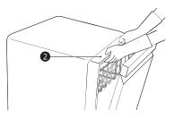
**1** Align the dishwasher with the opening. Make sure the water supply line and electrical cable are in the correct positions to slide into their channels properly.
