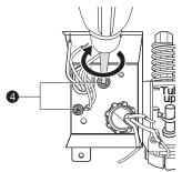
8 Pair the white, black, and green wires to the matching colored wires from the dishwasher. Then twist on the provided wire nuts ③ tightly to connect the corresponding wires.
