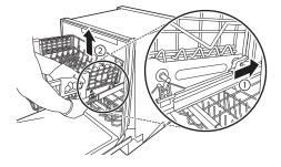
4 To replace the rack, place the back rack supports behind the rear hooks and pull the rack forward to snap the supports into the hooks. Then align the front rack supports with the front hooks and push the front of the rack down to snap the supports into the front hooks.
