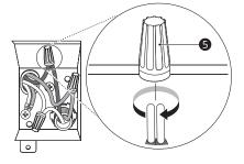
**9** Wrap electrical tape **()** around each connection.
