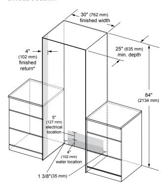
\*A minimum 4" (102 mm) finished return that matches the cabinet exterior is recommended on all sides and the top of the cutout opening. The shaded area will be visible after installation.
